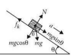
When the angle of inclination  $\theta$  reaches 30°, the block just slides,
