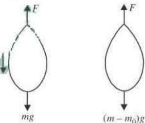
Let mass  $m_0$  be removed from the balloon so that it starts moving up with an acceleration a. Then,
