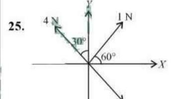
Three forces acting on a body are shown in the figure. To have the resultant force only along the y-direction, the magnitude of the minimum additional force needed is
